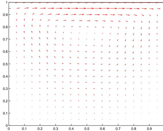
Figure 3: Velocity streamlines for  $Re = 1$ .
