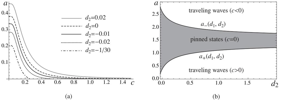
**Figure 5.** (a) The relation  $a(c)$  at  $d_1 = -0.2$  and different values of  $d_2$ . (b) The regions of existence of traveling waves and pinned equilibrium states at  $d_1 = -0.2$  for  $d_2 \geq -1/30$ .
