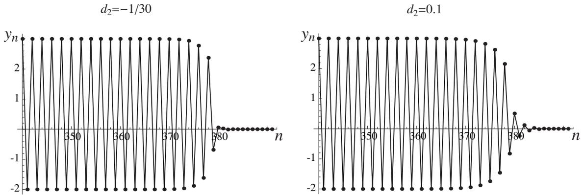
**Figure 6.** Snapshots of numerical solution of (2.1), (2.3) (circles) and traveling wave solution (lines) at  $t = 600$  corresponding to  $c = 0.15$ ,  $d_1 = -0.2$  and different values of  $d_2$ . Here  $a \approx 0.058$  at  $d_2 = -1/30$  and  $a \approx 0.508$  at  $d_2 = 0.1$ . The numerical simulations were run with these values of  $a$  and the initial condition given by  $\mathbf{u}_m(0) = (y_{2m}(0), y_{2m+1}(0)) = (\varphi_1(m - 100), \varphi_2(m - 100))$ .
