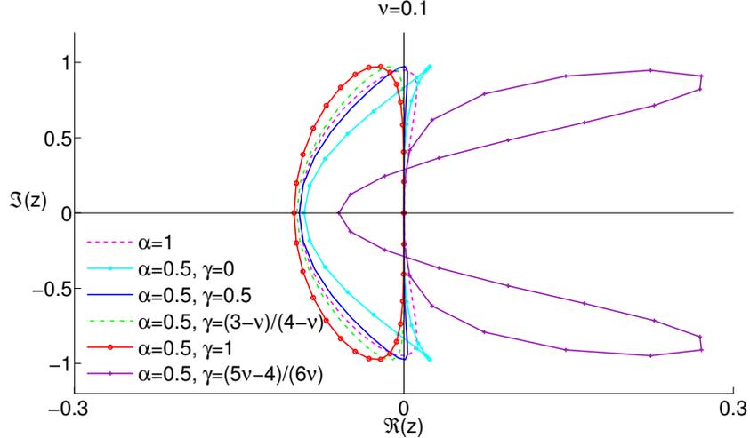
Fig. 2.1: Root locus curves for the scheme (2.2)–(2.4) are plotted for the case  $\nu = 0.1$ , for various combinations of  $\alpha$  and  $\gamma$ . Note that  $\alpha = 1$  corresponds to the original Robert–Asselin filter.
