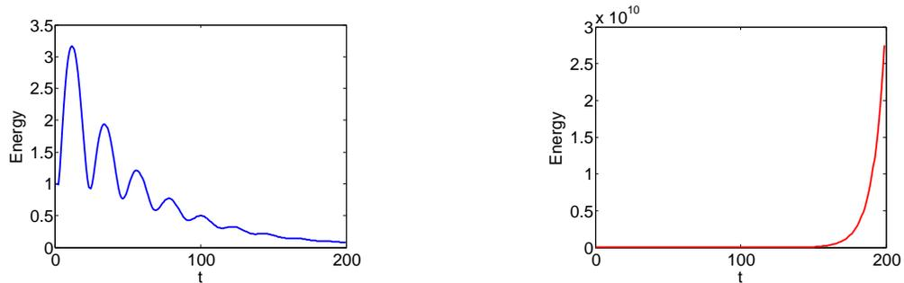
Fig. 3.1: Energy for the numerical solution of the scheme (2.2)-(2.4) with  $\Delta t = 0.99\delta t$  (left) and  $\Delta t = 1.01\delta t$  (right), where  $\delta t$  is the theoretical maximum stable time step derived in Section 2.3 for  $\alpha = 1/2$ ,  $\nu = 0.1$ , and  $\gamma = 0.5$ .
